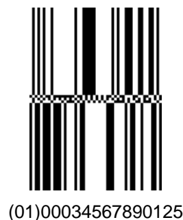
Abbildung 5.6.1.2.4 – 1 GS1 DataBar Stacked Omnidirectional Symbol
