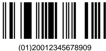
Abbildung 5.6.1.2.1 – 1 GS1 DataBar Omnidirectional Symbol
