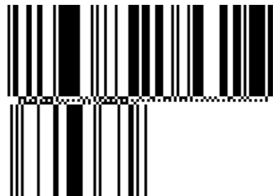
Abbildung 5.6.1.4.2 – 1: GS1 DataBar Expanded Stacked Symbol
